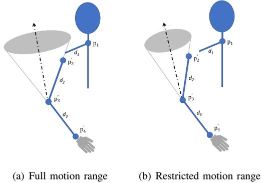
Fig. 3. Adaptation of the FABRIK solver with varying joint limits to optimize the REBA score of the posture associated to a desired end-effector pose.
