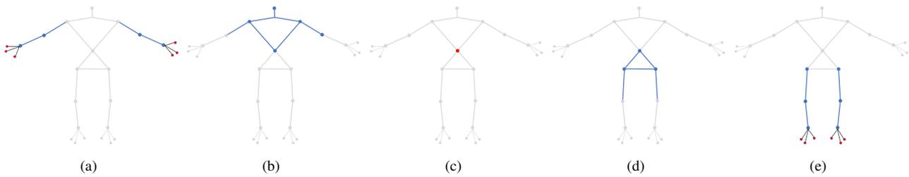
Fig. 4. Humanoid model: the different part of the body in a hierarchical fashion. The whole body movement is controlled in this order: (a) hand chains, (b) upper body triangle, (c) sub-base, (d) lower body triangle, (e) feet chains.
