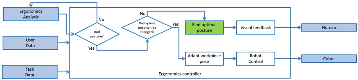
Fig. 2. Ergonomics controller scheme. Based on the ergonomics analysis and the task data (workpiece constraints) optimal postures are suggested to the user or the robot configuration is adapted. The algorithm described in this paper is highlighted in green in the diagram.
